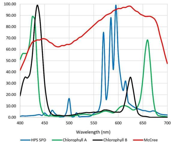
The spectral response of plants to optical radiation is a very complex topic. Many articles have been written about how 450 nm blue and 660 nm red LEDs are optimal for plant photosynthesis because these wavelengths correspond with the absorption peaks of chlorophyll A and B photopigments. However, these represent the absorption of chlorophyll extracts dissolved in a solvent such as ethanol. Many other components in the plant leaves interact with the absorbed light.
